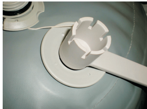
Cap off, ready to remove valve.
