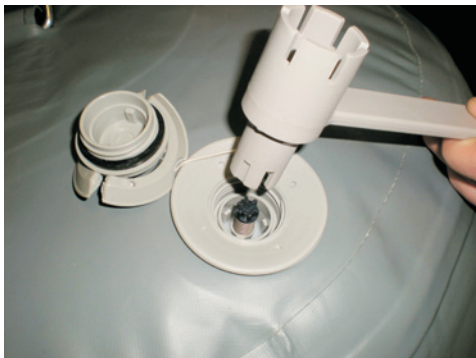
Wrench in valve ready to remove.
